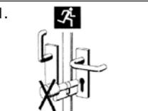
No lock with lock cylinder with a thumbturn or rotary knob should be fitted to emergency doors
