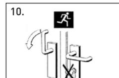
No key should be left inserted in locks on emergency doors.
